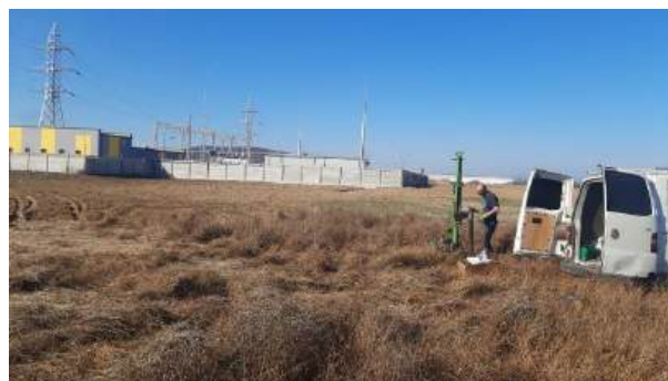
Fig. 10. Execution of borehole FS04+DPH
